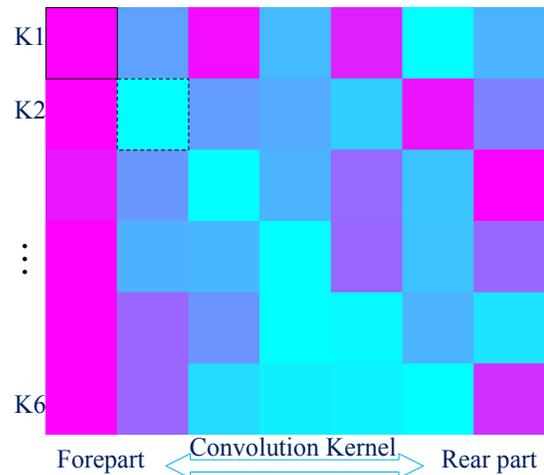
Figure 4: Visualization of convolutional kernels from the first convolutional layer (better viewed in color and rows). Each row represents a convolution kernel of size 7 and there are kernels (termed K1, K2,  $\dots$ , K6) from 6 feature maps. Colors varying from bright blue (dashed line box) to bright red (black box) map values from low to high, representing response intensity of kernels with respect to input.
