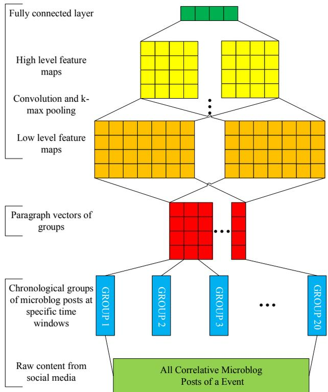
Figure 2: The framework of CAMI. From the bottom up: split raw content into chronological groups based on the distribution; learn paragraph vectors for all groups; extract features from low level to high level with CNN.
